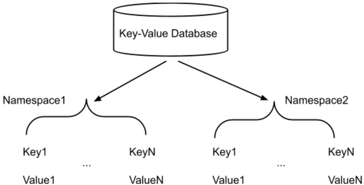
Bitcoin node uses LevelDB as a database to store block and transaction information. LevelDB is a key-value database, so it is convenient to also use it to store our newly introduced key-value pairs.
